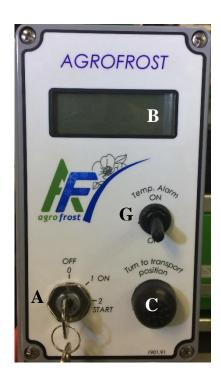
A <u>main switch / key</u> With this switch the FrostGuards engine can be started or turned off.
