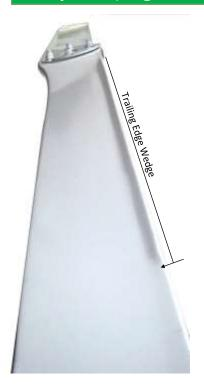
The Chinook blade is constructed from composite fiberglass; machine made into on piece. The blade, with steel teeter hub attached, weighs only approx. 45 kg. This low weight and one piece form provides for smooth running, vibration-free operation.
