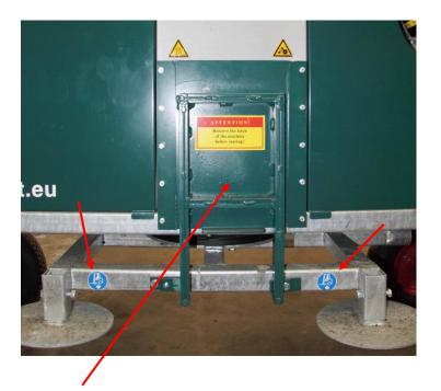
The cover plate for the fan outlet prevents the FrostGuard of turning around during transport. (GC20)
