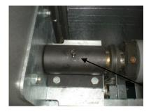
Every 15 working hours, the bearing of the transmission shaft at the centre of the machine has to be greased.
