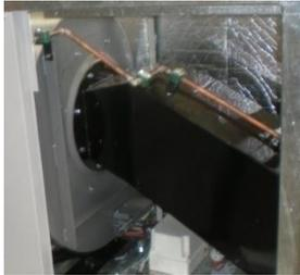
Ventilateur avec brûleur : the fan uses the rotational energy received from the engine to move large quantities of air. By using the heat energy provided by the built in burner ring, the FrostGuard heats up the air it displaces.
