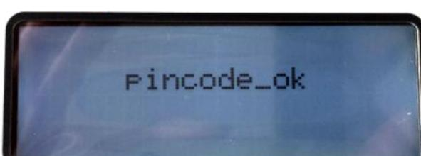
The PIN-code remains in the memory and has to be reinstalled only when you use another SIM-card with a different PIN-code. Once the PIN-code is set, the alarm will not ask for it again during a next start up.
