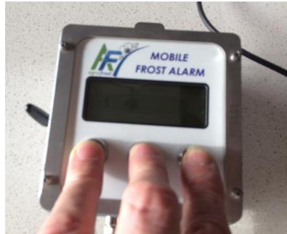
**We advice to reset the alarm when you connect the alarm with the battery for the first time.**
