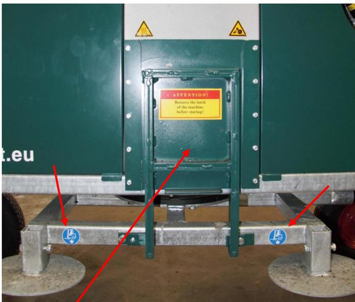
The cover plate for the fan outlet prevents the FrostGuard of turning around during transport. (GC20)
