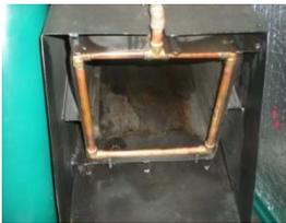
Side outlet of the fan (GC20): this outlet ensures laminar flow. It is not possible to protect this outlet more without influencing the initial operation of the machine. Therefore a residual risk remains.
