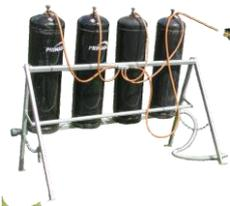
Gas cylinders: the machine makes use of the combustible gas these cylinders provide to heat up the air. They need to be installed on the gas bottle holder that is provided with the FrostGuard. It is important that the gas bottle holder is attached with the machine via the silencer and the exhaust pipe.
