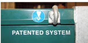
Fixing/ Lifting eye: you have to use this tool for fixing the machine firmly during transport. You have to use all these eyes at both sides of the machine if you want to hoist the machine.
